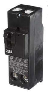
Siemens Low Voltage Residential Circuit Breakers Main Breakers -Branch Main Breakers Non-reversible are Circuit Protection Load Center Mains, Feeders, and Miniature Circuit Breakers. Type: QN Application: Electrical Distribution Standard: UL 489 Voltage Rating: 120/240V Amperage Rating: 175A Trip Range: Thermal Magnetic Interrupt Rating: 10 AIC Number Of Poles: 2P
