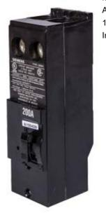
Siemens Low Voltage Residential Circuit Breakers Main Breakers - Branch Main Breaker Reversible are Circuit Protection Load Center Mains, Feeders, and Miniature Circuit Breakers. Type: QNR Application: Electrical Distribution Standard: UL 489 Voltage Rating: 120/240V Amperage Rating: 175A Trip Range: Thermal Magnetic Interrupt Rating: 10 AIC Number Of Poles: 2P
