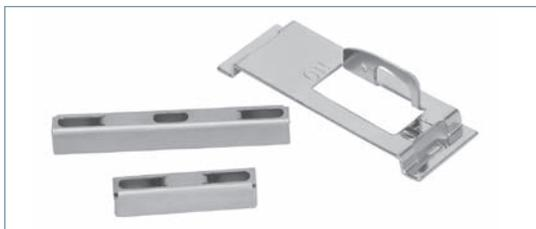
**BOD and NGB, HGB, LGB handle ties** are now released for use where single pole breakers are using shared neutrals and must be locked out simultaneously.
