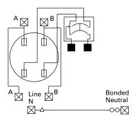
Wiring Diagram Key ○ #14-2/0 AWG △ #14-2 AWG
