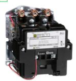
NEMA Contactor, Type S, nonreversing, Size 3, 90A, 50 HP at 575 VAC, 3 phase, up to 100 kA, 3 pole, 120 VAC coil, open
