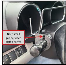
STEP 6 – Check SAFEDRIVE signal arm for level, bend as necessary
