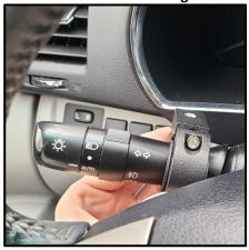
STEP 5 – Install SAFEDRIVE signal arm and tighten set screw
