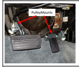
Remove the brake pedal PulleyMount and the gas pedal PulleyMount (if you have the SafeDrive Pro Plus) from the pedals.
