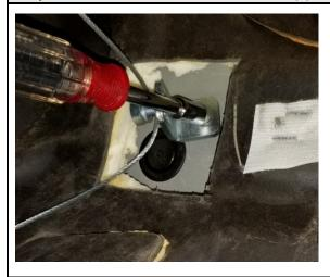
Release the steel cables from the QuickConnect behind the pedal(s) on the vehicles left side.
