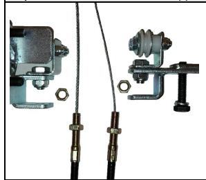
The goal of this step is to remove the black conduit cables from the hardware so it can be replaced.
