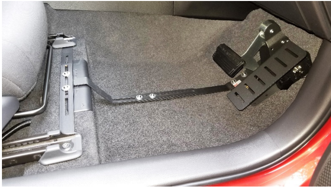
*This picture shows the T-Mount modified with bends for a custom fit
