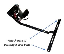
The T-Mount is an optional add-on to the SafeDrive Pro or SafeDrive Pro Plus to avoid the need to bolt the pedal system into the passenger side floor. The SafeDrive T-Mount is secured using the passenger side front seat bolts which attach the seat to the car. It is fully adjustable and is made with a thick enough steel to ensure stability and allow bending to shape for a custom install. The SafeDrive T-Mount connection points are already threaded to fit the included screws and hand bolts.
