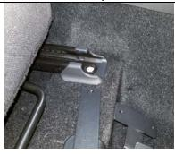
2. Slide the leg of the T under the top of the two T parts which were installed to the seat bolts.
