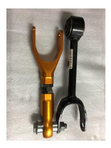
Now turn the turnbuckle until the arms are the same length to the center of the bolt holes. With the arms the same length tighten down the lock nuts. Now you can install the arms in the car.
