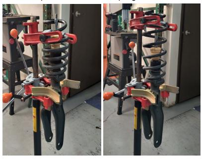
Place the stock shock in your spring compressor to hold the spring tension.
