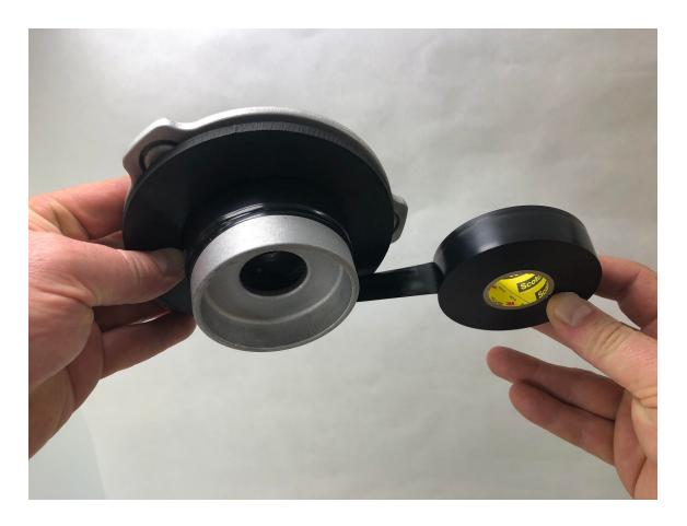
• With the tophat installed, addl the short damper shaft spacer in the upper recess on the OEM top hat.
