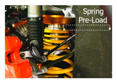
threads to start, and add to additional threads as you move the adjuster If you plan on lowering the car further.
