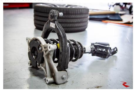
**Step 3:** Remove the stock upper control arm by removing the 2 13mm bolts that secure the arm to the carrier.
