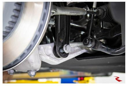
• With the previous parts removed, we will go back to the top of the front shock tower to prepare to remove the shock, upper control arm, and the carrier as one assembly.
