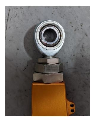
With all the treads all the way in you will then hold on to the arm and turn the rod ends the shortest direction so that the holes through the rod end are in the same plane as the arm as shown.
