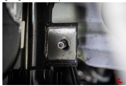
• Using a torx bit, undo the pinch bolt attaching the front knuckle to the upper control arm. Remove the bolt and tap up on the control arm to get the upper ball joint out of the socket in the front knuckle.
