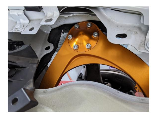
Now that you have ensured that there are a couple mm at least in between the tip of the arm and the chassis you can use the provided zip ties to secure the grommets on the wheel speed sensor to the arm, and re attach the ball joint to the upright.
