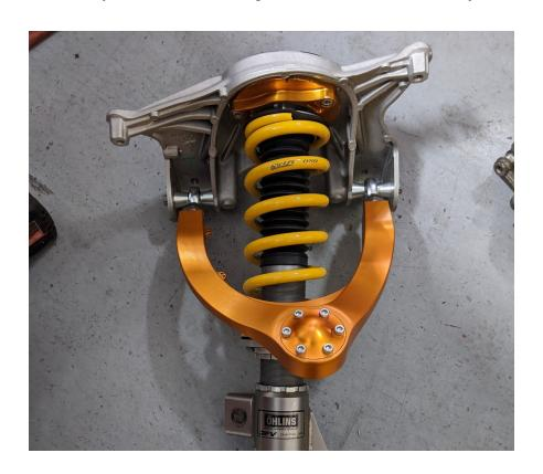
**Step 6:** Reinstall the arm/carrier/shock assembly into the car. This is simply the reverse of removal with a couple small changes. First, the arm is a tempting handle to lift the suspension by, but there is now a pinch point in between the arm and the carrier because of the switch from rubber bushings to spherical rod ends so be wary of lifting by just the arm.
