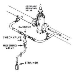
Injector installed around a point of restriction such as a regulator valve or gate valve which creates a differential pressure, thereby allowing the injector to produce a vacuum.
