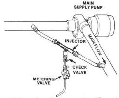
Injector installed across the differential pressure created by an existing booster or supply pump in the system. It is plumbed from the discharge side to the intake side of the pump.
