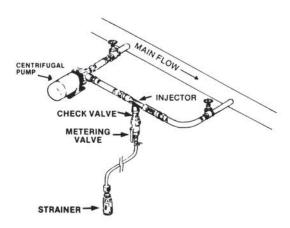
Installed in conjunction with a centrifugal pump to boost pressure through the injector thereby creating a differential pressure and producing a vacuum for chemical induction downstream from the pump.
