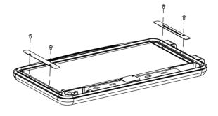
2) Take out the glass, and check if the grey rope beneath needs replacing. If so, replace this rope as well.
