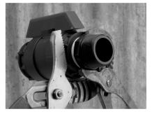
3. Using a pipe wrench or multigrips on the end caps only, further screw the blue handled ball valve into the male thread until tight. Where necessary ensure the male thread is held stationary to avoid it from moving. Do not use pipe wrench or multigrips on the body of the blue handled ball valve.
