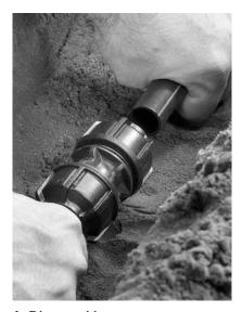
6. Disassembly To disassemble the fitting simply loosen the nut using a wrench until 2 threads are showing. Pipe will be released and can simply be pulled out of the fitting.
