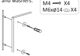
5. Flip the vanity over and attach each foot with 4 M4X20 screws.
