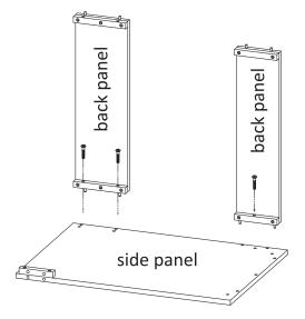
2. Tighten down the bottom of the vanity with the M6 bolts.
