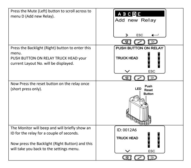
The New Layout has now been saved to the Monitor and Relay and you can now program in the new sensors.
