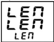
As long as enter this mode, insert battery into 'learnable sensor' immediately, the LCD monitor will beep once and finish learning process.
