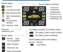
This TPVMS except tire pressure, temperature detection, also with the tire abnormal vibration detection function, which may reconnaissance vehicle tires other abnormal phenomena, can also become a tool for more warning function
