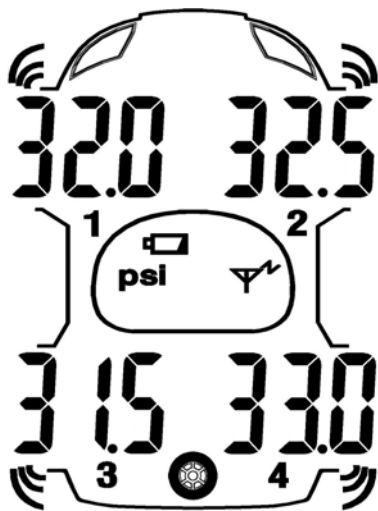
Low Monitor Battery Indicator
