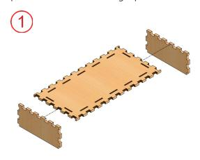
Slide side plates into the top plate.
