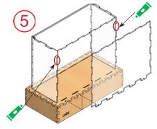
Insert Front plexiglass part into the slots. Apply glue on top at connection points to hold parts in place
