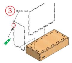
Remove masking tape from both sides of plexiglass parts. Insert Back and Left side parts into the slots. Apply glue on top at connection points to hold parts in place
