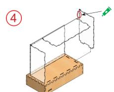
Insert Right side plexiglass part into the slots. Insert top cover into holes of side plates before applying glue on top at connection points.
