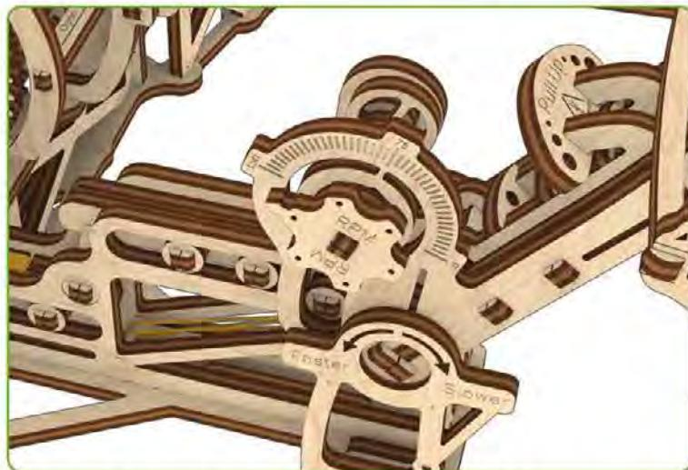
**ENG** «RPM Module» The maximum speed limit of the engine is limited in the form of an sheave. With the knob on the «0» mark, the engine speed is reduced to the minimum speed, and when the handle is at the «150» mark, the engine speed is reduced to the maximum engine speed. By adjusting the «RPM Module» handle, you can achieve the ideal engine speed for each of the proposed aircraft models.
