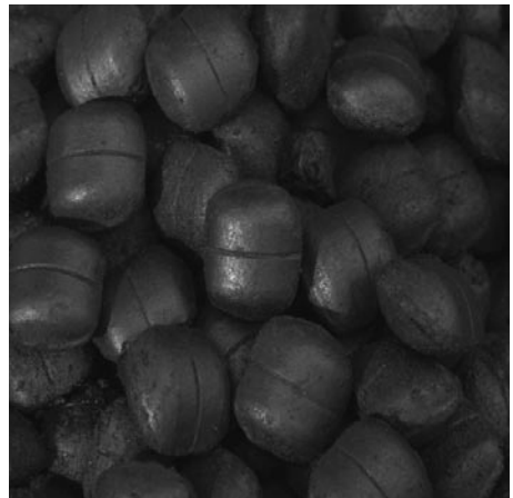
The recommended maximum fuel load for Approved Smokeless Coal is approximately 1.5kg (just over 3lbs)
