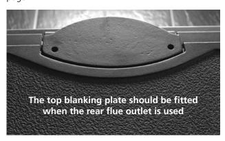
• Flue Outlet The Aidan Eco Boiler stove comes configured for a top flue outlet but also has a rear flue option. A shaped top flue collar is provided and there is a blanking plate for use on the top when using the rear flue. The connecting flue pipe size is 150mm (6") and should never be reduced.
