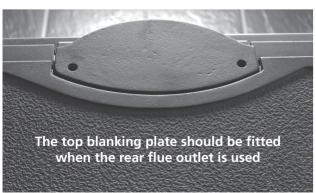
• Flue Outlet The Aidan Eco Boiler stove comes configured for a top flue outlet but also has a rear flue option. A shaped top flue collar is provided and there is a blanking plate for use on the top when using the rear flue. The connecting flue pipe size is 150mm (6") and should never be reduced.
