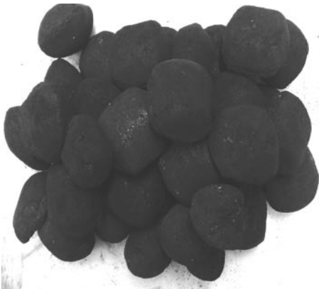
The recommended maximum multi fuel load: Photo shows a typical fuel load of approximately 1.75kg of approved smokeless ovals
