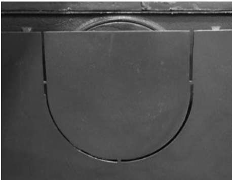
The Precision II pre-cut rear heat shield. When using the rear flue outlet option the cut out can be easily removed by using a junior hacksaw blade to cut through the 3 small retaining links.
