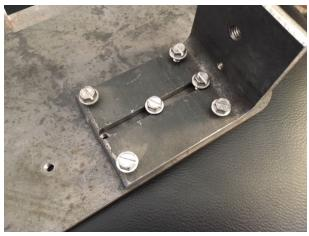
loosened to adjust for lateral alignment. The same bolts should also be loosened and the four corner bolts used to square up the tilt table to the flat platen of your grinder. This one time adjustment is then locked into position by tightening the center two bolts. Adjusting for squareness should be done without a belt in place on the flat platen.
