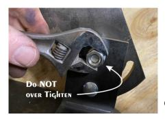
Do not over tighten the 3/8 nut. You want to be able to adjust the angle of the table with a little resistance from the lock washer compression. When lock handle is tightened table should be rigid.
