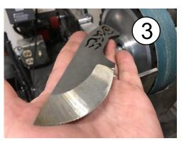
A finer grit belt can be used to polish the bevels.
