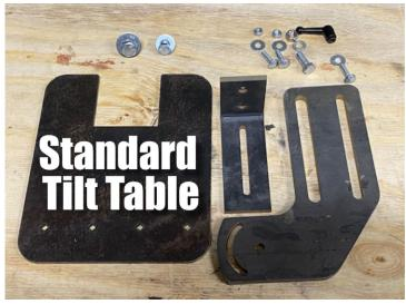
Step 2 Angle iron gets secured with two carriage bolts, washers and nuts. Pivot arm is secured with a 3/8 bolt, lock washer and nut. Locking handle screws into remaining carriage bolt.
