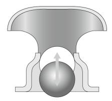
Pumps having a water jacket are equipped with this valve. The ball is made of steel or rubber and is located at the top of the water jacket.
