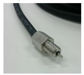
This time, we introduce the externally mounted leak sensors. They are the leak sensors that are installed in place of the oil plug, unlike the leak sensors that are built into the motor. There are 3 models, M8/10/12, depending on the size of the oil plug.
