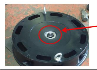
Labyrinth Ring on the upper pump casing of LH6110
