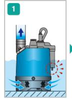
Pump continues to run while the electric probe remains submerged.
