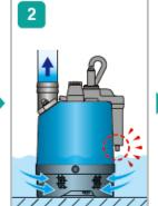
When the water surface falls below the electric probe, timer starts to count about one minute.
