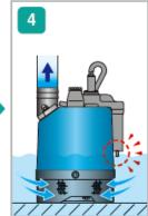
When the water level rises to contact the electric probe, pump starts operating again.
