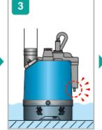
Pump stops in about one minute after the water level falls.
