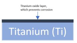
Therefore, even if this film gets mechanically damaged, the base Titanium forms a new oxide layer in no time, and maintains its corrosion resistive property. This provides Titanium with exceptional resistance to corrosion in extremely wide range of aggressive environments.
