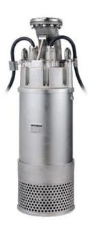
All the other features of standard LH series pumps, like center flange discharge, seal pressure relief port and top flow-through discharge for better cooling efficiency are also present in these fully stainless steel LH series pumps. Besides the metallic parts, all the rubber parts, like O-ring, oil seal and mechanical seal, have been upgraded to FPM (FKM) material for higher resistance to chemical.
