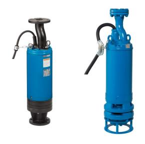
"Tandem operation" is an operation method that connects two pumps of the same model in series. This provides double pump head at the same flow rate in comparison with that of a single pump. The principle of tandem operation is the same as that with multistage pumps. The LH and LH-W series pumps adopt the center flange construction to align the discharge pipe with the cylindrical pump center axis.
