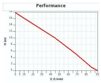
Characteristics referring to operation with water at 20  $^{\circ}$
