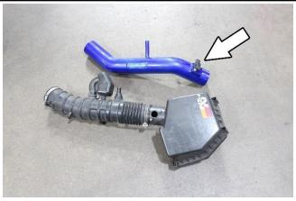
19. Remove and install the mass air flow sensor onto the HPS intake pipe using the provided M4  $\times$  8mm allen bolts.
