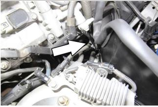
18. Loosely secure the provided intake bracket onto the vibration mount with the angled side pointing upwards.
