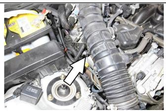
6. Unclip the fuel hose from the intake tube.
