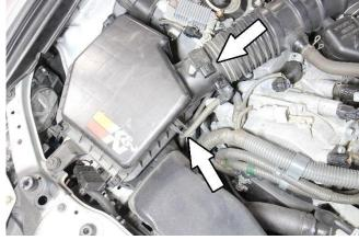
4. Disconnect the mass air flow sensor and unclip the harness from the upper air box.
