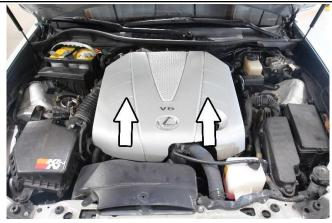
3. Lift to remove the engine cover from the vehicle.
