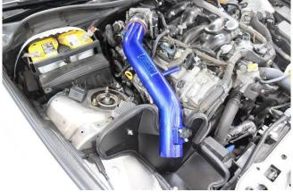
20. Insert the HPS intake pipe into the throttle body coupler and secure the intake pipe to the intake bracket using a M6x12mm bolt and washer. Once the intake pipe is moved into the proper position, tighten down the T-bolt clamps and the intake bracket.
