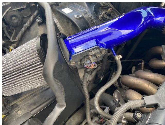
17. Reconnect the MAF sensor harness.
