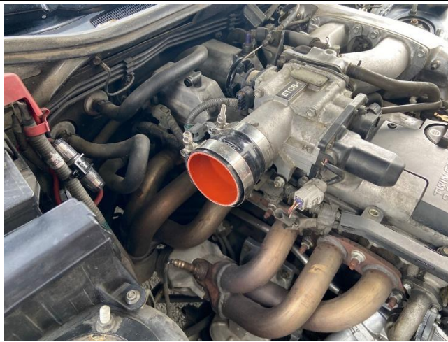
9. Insert the reducer coupler onto the throttle body along with the provided T-bolt clamps.
