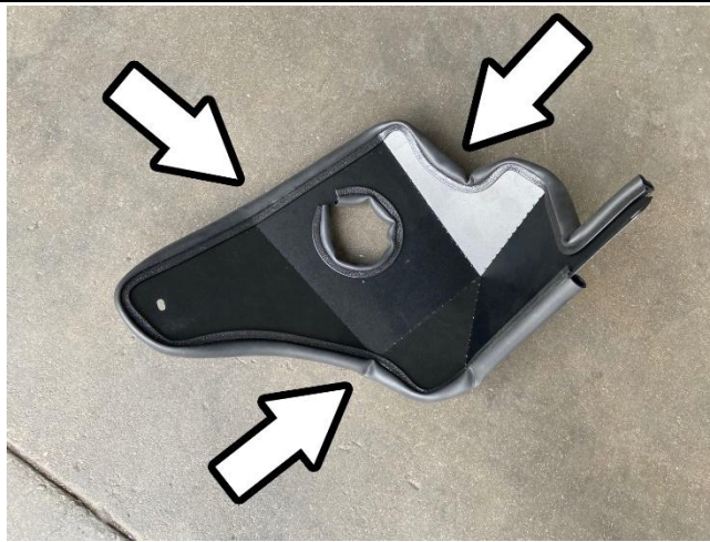
10. Install the provided bubble edge trim onto the heat shield.
