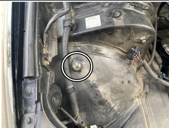
11. Install the provided 1/2" vibration mount onto the factory airbox mount.
