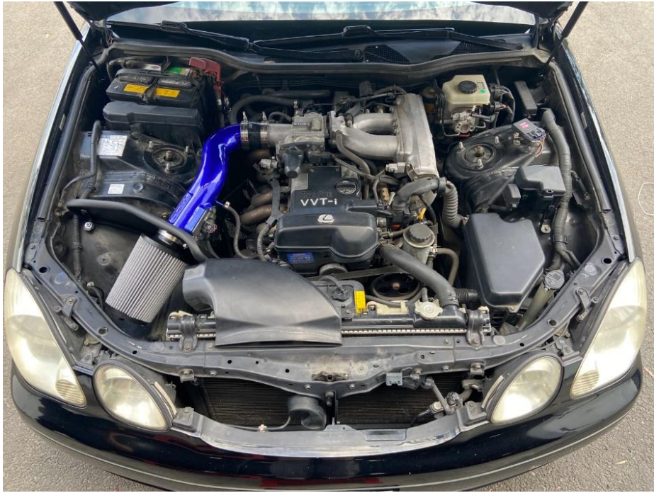
HPS Performance Air Intake Kit with Heat Shield (827 Series) 1998-2000 Lexus GS300 3.0L Part Number: 827-705
