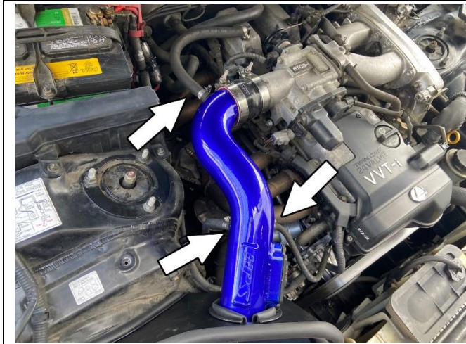
15. Insert the HPS intake into the heat shield and into the throttle body. Next, install and secure the EPDM hoses onto the intake pipe.
