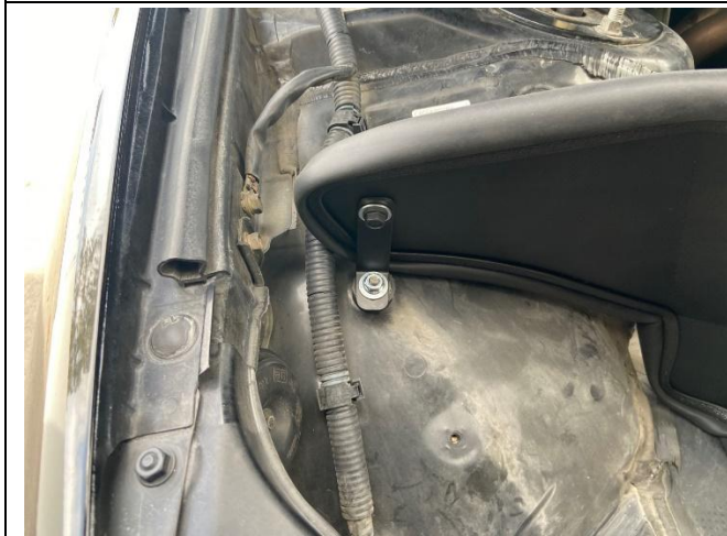
13. Fasten the provided "L" bracket onto the heat shield and vibration mount using the M6x16mm bolt, washers, and nuts.
