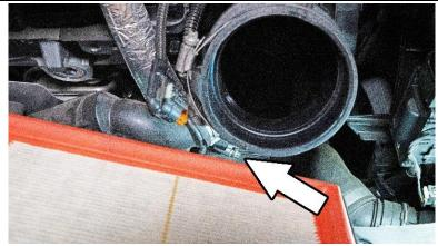
7. Loosen the hose clamp securing the intake hose from the turbo inlet housing.
