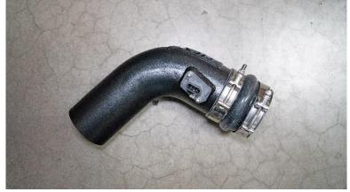
14. Insert the HPS hump coupler onto the sensor side of the HPS intake pipe with the provided T-bolt clamps.
