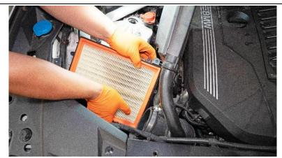
8. Lift up and pop the lower air box from its mounting grommets and disconnect the hose from the turbo inlet housing then carefully remove the assembly from the engine bay.
