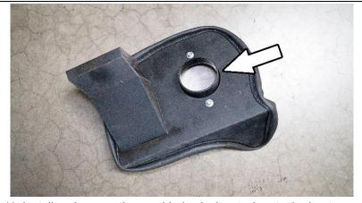
11. Install and secure the provided velocity stack onto the heat shield using the M6 x12mm bolts and washers.
