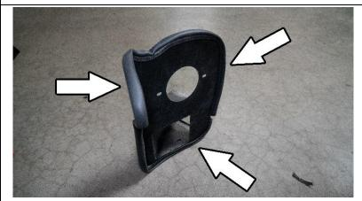
10. Install the provided bubble edge trim onto the HPS heat shield.
