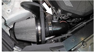
20. Insert and fasten the HPS performance air filter to the velocity stack. Reconnect the sensor.
