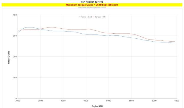
HPS Performance Air Intake Kit with Heat Shield (827 Series)
