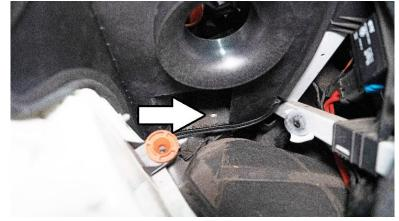
17. Secure the heat shield onto the M6 bung using the provided M6x12mm bolt and washer.
