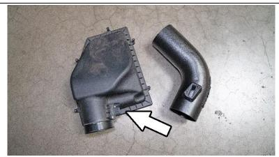
13. Transfer and secure the sensor onto the HPS intake pipe using the provided M4 bolts.
