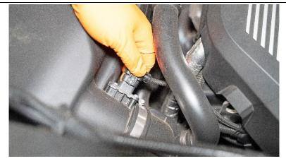
3. Disconnect the sensor electrical harness connector.
