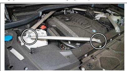
2. Remove the passenger side strut tower brace using a E12 and 18mm socket.
