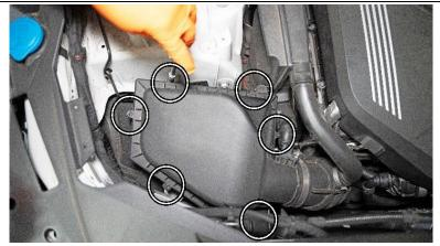
4. Loosen the 6 bolts securing the upper air box assembly using a T25 torx bit.
