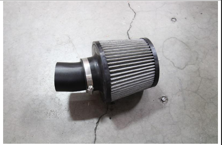
18. Insert the HPS performance air filter onto the HPS intake pipe.
