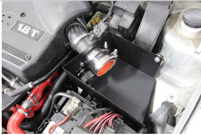
17. Install the 2.75" coupler onto the MAF housing along with the provided T-bolt clamps.
