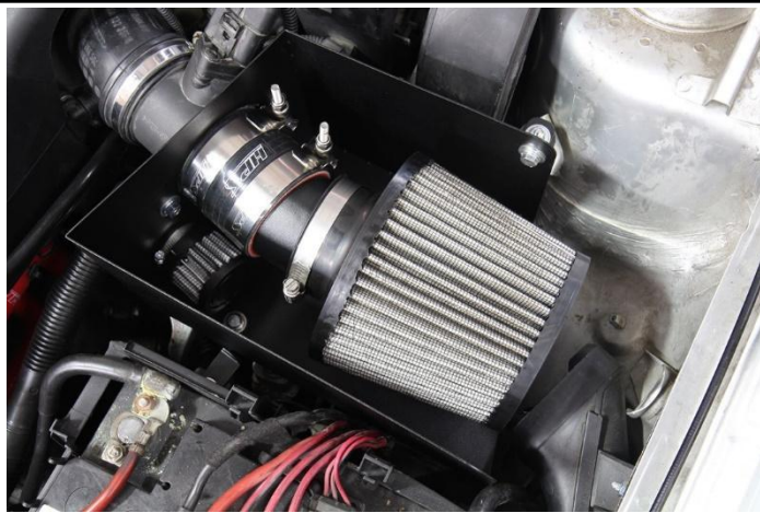
19. Insert and secure the HPS intake pipe into the coupler.
