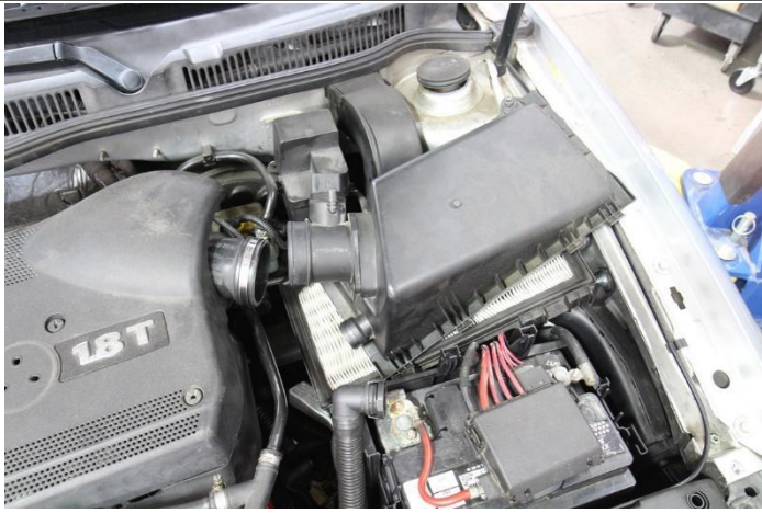
5. Remove the upper air box assembly from the vehicle.
