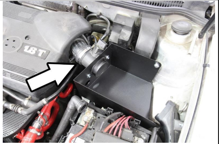
12. Re-insert and secure the MAF sensor housing back into the factory intake tube.
