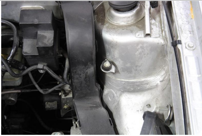
11. Insert the provided vibration mount onto the factory air box mount.
