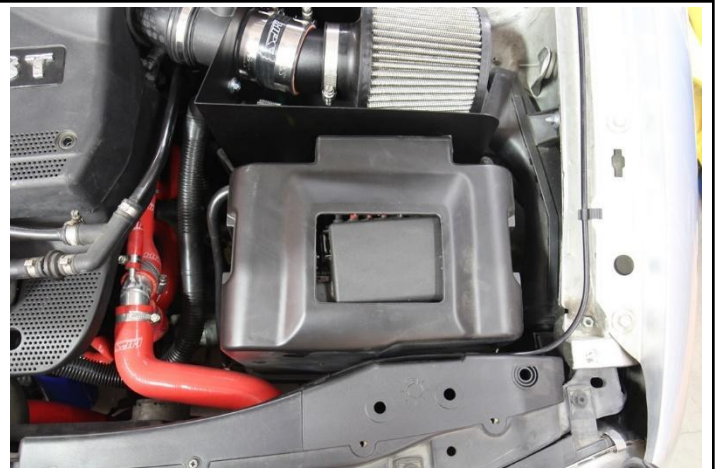
20. Re-connect the negative battery terminal and install the battery cover.
