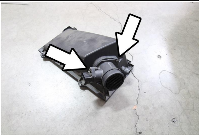
7. Loosen the screws securing the MAF sensor housing to disconnect it from the upper air box.
