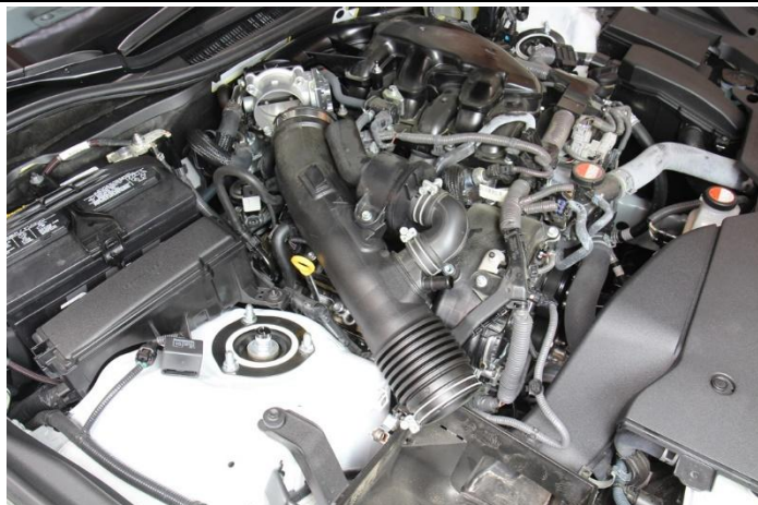
10. Disconnect the stock intake tube from the throttle body and remove it from the vehicle.
