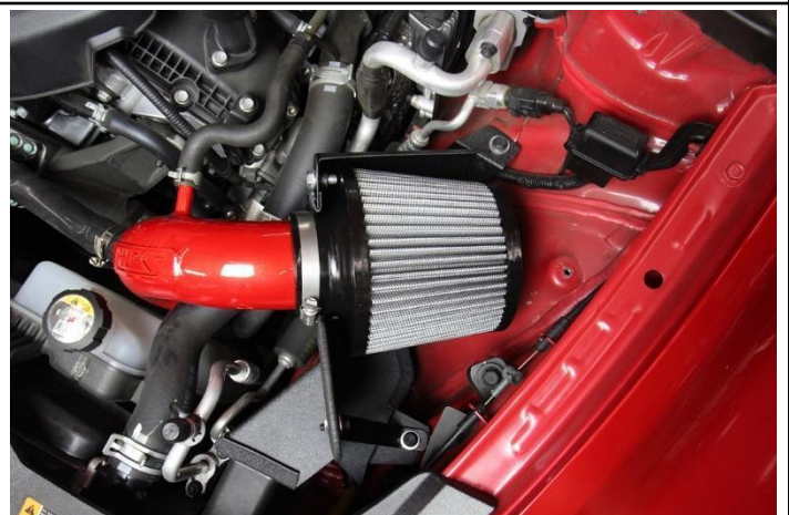
27. Install the provided HPS performance air filter.
