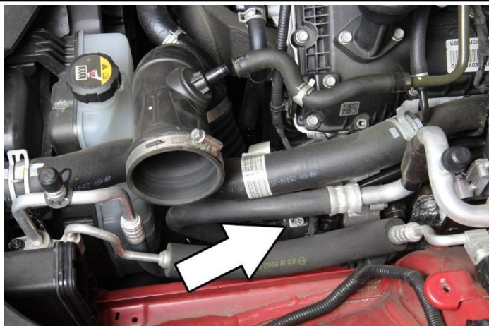
14. Loosen the clamp securing the intake tube from the turbo inlet.
