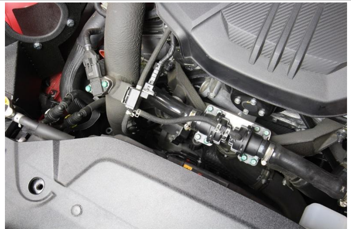
33. Insert and secure the remaining hose onto the BOV outlet with the provided hose clamp.
