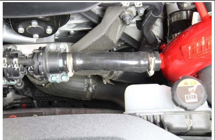
25. Insert the hose into the BOV outlet and secure the hose with the provided hose clamp.
