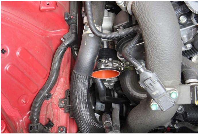
28. Install the coupler along with the provided clamps onto the passenger side turbo inlet.
