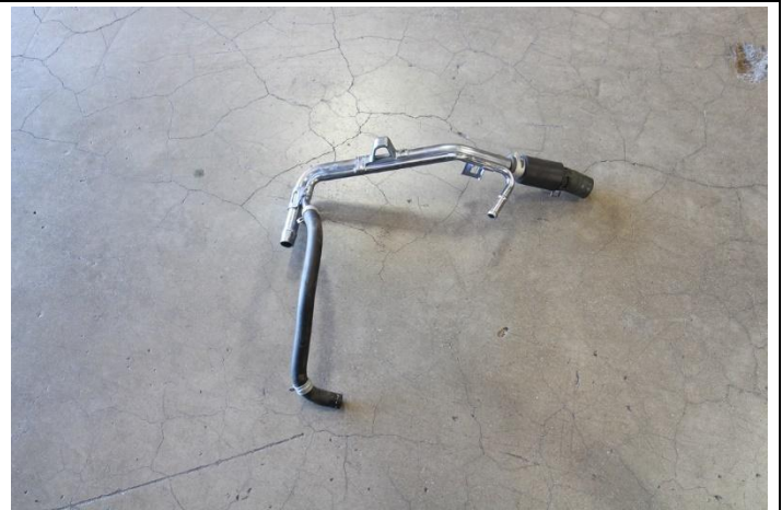
11. Remove the breather and coolant hard line assembly from the vehicle.
