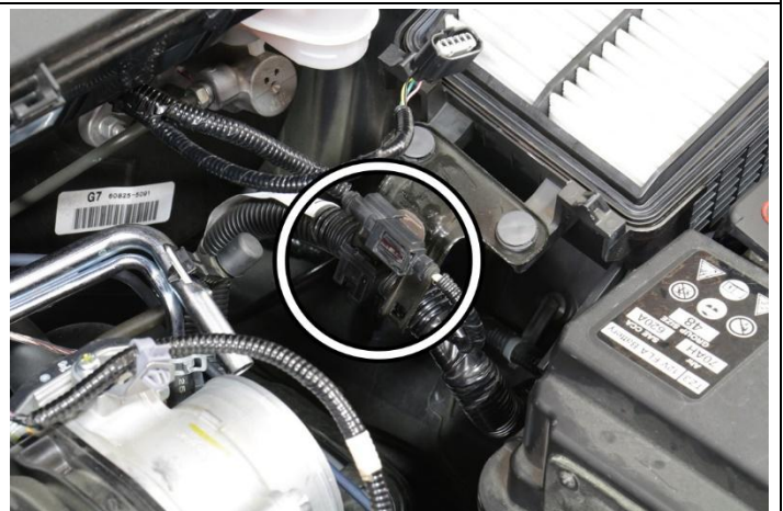
7. Depress each latch and remove the wiring harnesses from the air box bracket.
