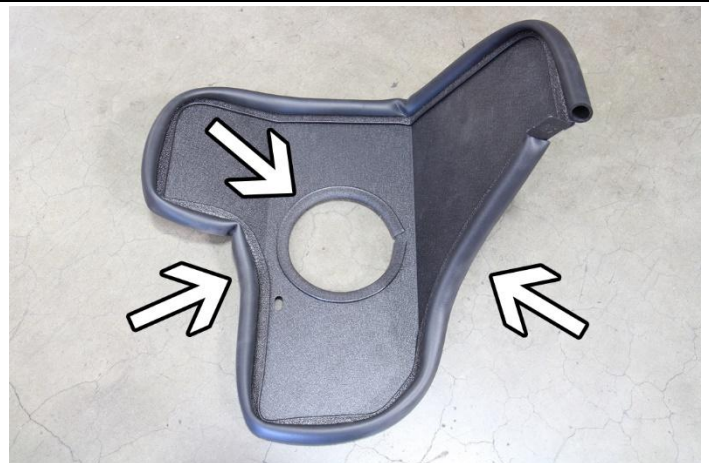
19. Install the bubble edge trim on the outer part of the heat-shield and the thin edge trim onto the opening of the heat-shield.
