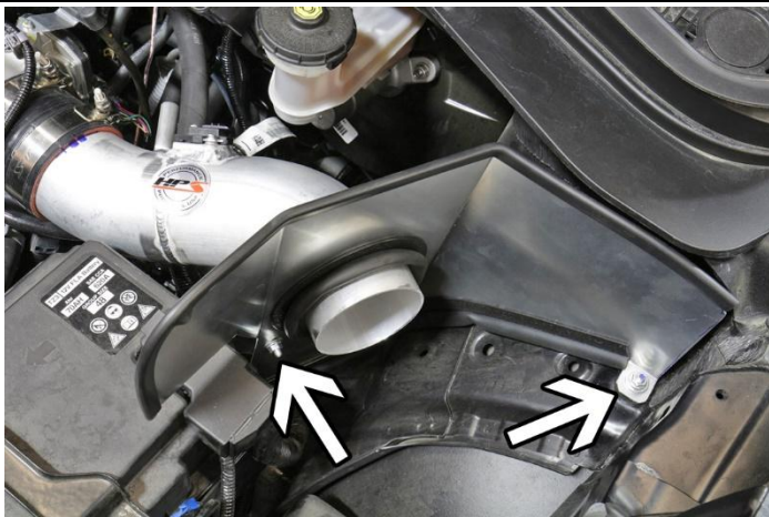
22. Insert the intake into the heat-shield. Secure the heat-shield onto the bracket and the vibration mount using the remaining M6x16 bolt, nuts, and washers. Once secured, position the intake to the proper position and secure the intake pipe.
