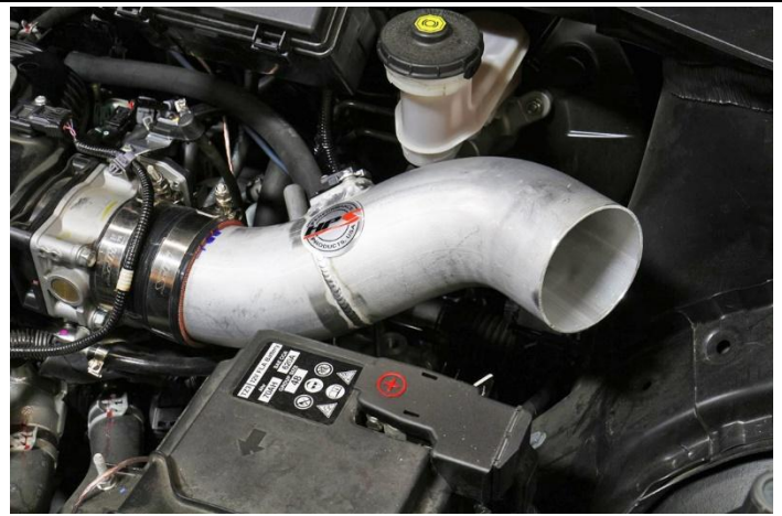
21. Insert the HPS intake into the reducer coupler, but do not secure the intake yet.
