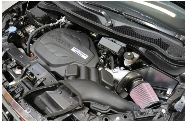
25. Re-install the air duct and the engine cover back onto the vehicle.
