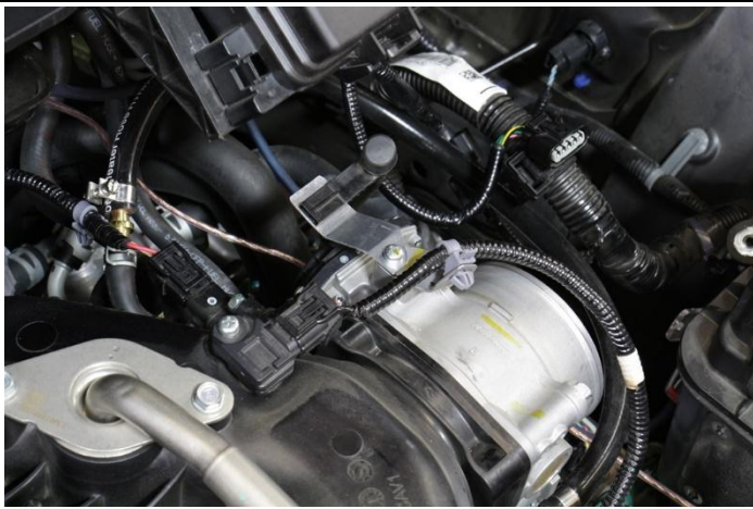
14. Re-using the screw removed from the previous step, install the provided bracket on top of the harness bracket. Install the transmission breather hose onto the bracket.
