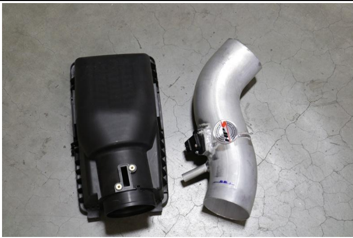
20. Install the Mass Air Flow sensor onto the HPS intake.
