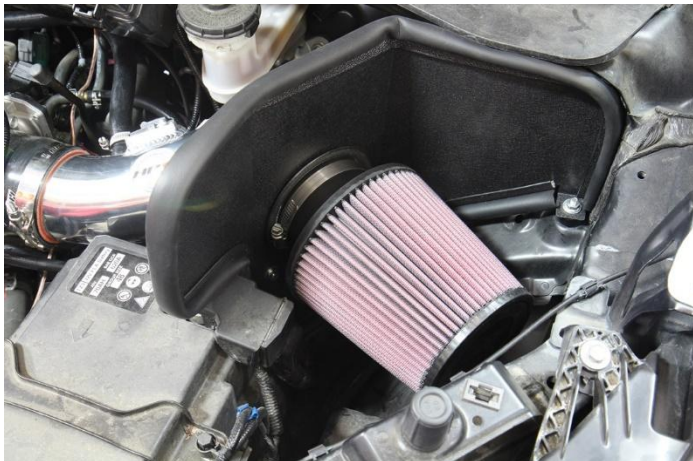
24. Install the provided HPS filter onto the HPS intake pipe.
