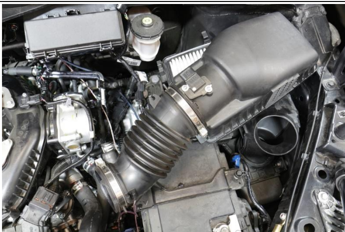
6. Remove the stock intake tube along with the top portion of the air box from the vehicle.
