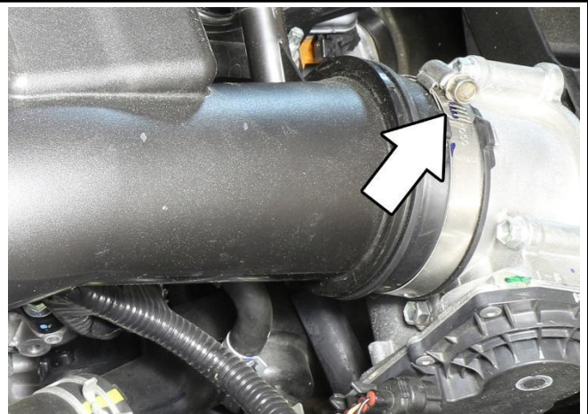
7. Loosen the hose clamp and remove the air intake tube from the throttle body.
