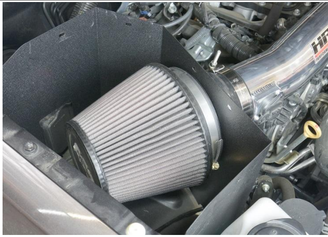
22. Install the HPS air filter onto the velocity stack and secure it using a flat head screwdriver.
