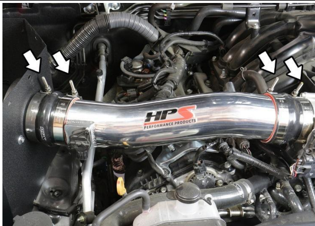
26. Rotate and position the T-bolt clamps to your desired position so as to not obstruct any surrounding items.
