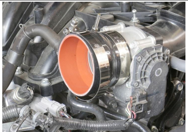
15. Install the silicone reducing coupler onto the throttle body. Secure it to the throttle body using the smaller T-bolt clamp.
