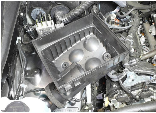
10. Remove the air box base from the engine bay.
