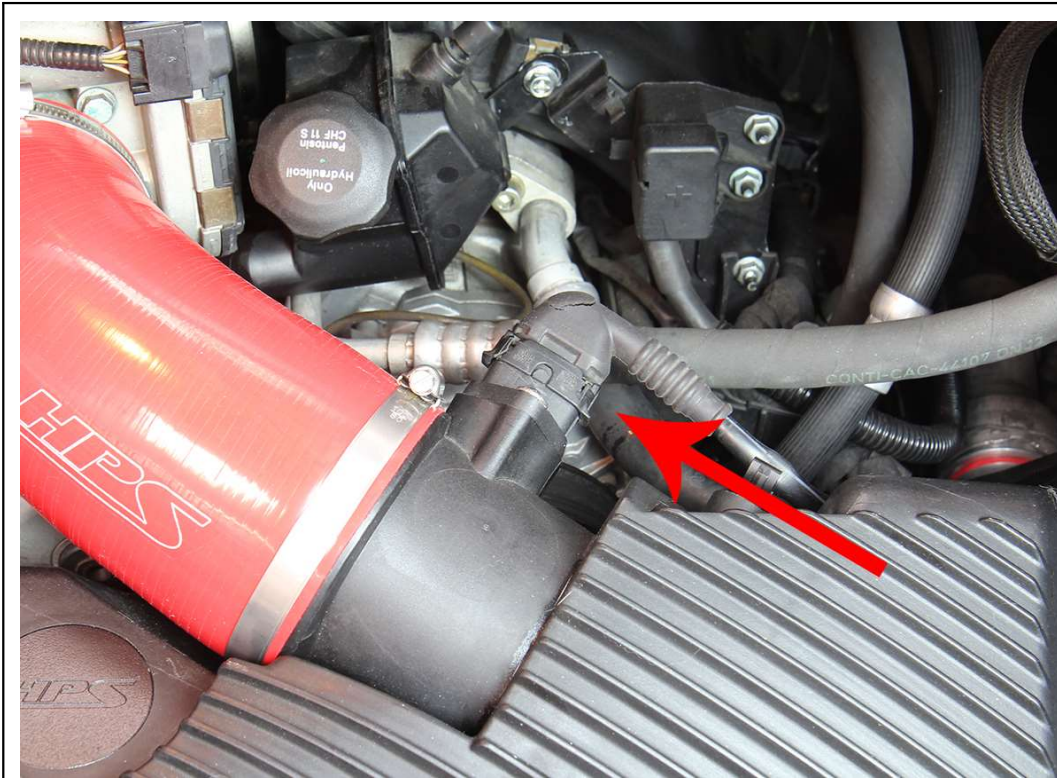
19. Reconnect the MAF sensor.
