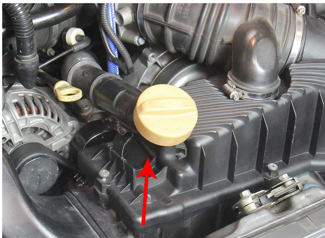
4. Unclip oil fill neck from the air box.
