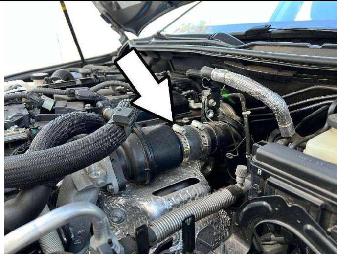
9. Loosen the hose clamp securing the intercooler hose from the turbo resonator.
