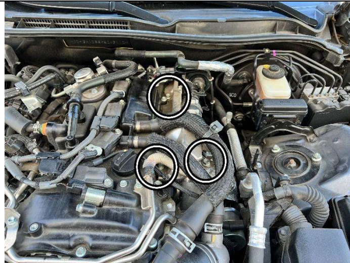
7. Remove the 3 bolts (2x 12mm, 1x 10mm) securing the heat shield.
