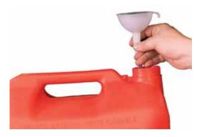
If you have been using gasoline in your water pump, before storing your water pump for extended periods of time you should drain your engine fuel tank of gasoline.
