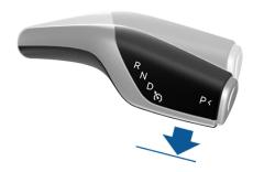
Note: When Traffic-Aware Cruise Control cancels, Model Y does not coast. Instead, regenerative braking slows down Model Y in the same way as when you move your foot off the accelerator when driving without Traffic-
