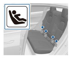
In the second row, install LATCH child safety seats in the outboard seating positions only. Use only a seat belt retained seat in the center position.
