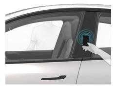
Once inside, power up Model Y by pressing the brake pedal within thirty seconds of scanning the key card (see Starting and Powering Off on page 56). If you wait longer than thirty seconds, you must re-authenticate by placing the key card near the card reader. located behind the cup holders on the center console. When your key card is detected, your 30 second authentication period restarts.
