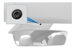
Keep the camera lens clean, and free of obstructions. Remove any buildup of dirt or dust by occasionally wiping the camera lens with a soft damp cloth.
