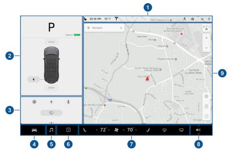
1. This area on the top of the touchscreen displays useful information and provides shortcuts to various features. In addition to the time of day and the current outside temperature, this area displays the following icons:
