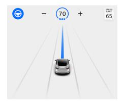
When Navigate on Autopilot is active and you approach an off-ramp or freeway interchange along your navigation route, the appropriate turn signal engages and Autosteer maneuvers Model Y onto the off-ramp or interchange.
