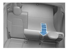
**Note:** Before folding seats fully forward, remove any items from the seats and the rear footwell. To allow the seat backs to fold completely flat, you may need to move the front seats forward.
