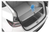
Caution: Never load more than 130 lbs (60 kg) on the rear load floor (above the lower trunk compartment) or more than 285 lbs (130 kg) in the lower trunk compartment. Doing so can cause damage.
