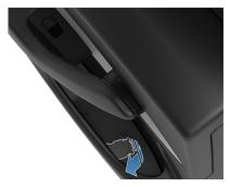
Pull the mechanical release cable (foam block) to release the door latch.
