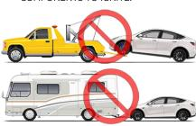
Do not transport Model Y using any method that is not specified by Tesla. Adhere to the instructions provided in the following sections and observe all warnings and cautions provided. Damage caused by improper transporting of your vehicle is not covered by the warranty.
