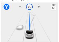
If Require Lane Change Confirmation is turned off, Navigate on Autopilot engages the appropriate turn signal, checks for vehicles and objects, and when appropriate. maneuvers Model Y into the adjacent lane.
