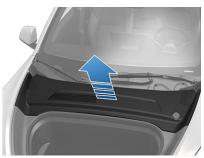
3. If checking the Battery coolant, remove the cabin intake trim panel by pulling it upwards to release the clips that hold it in place.
