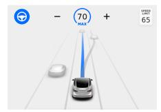
When the touchscreen displays a message asking you to confirm the lane change, engage the appropriate turn signal. If you do not confirm the lane change within three seconds, a chime sounds to remind you that Navigate on Autopilot requires your confirmation to change lanes.
