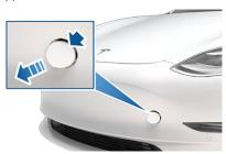
Fully insert the tow eye into the opening, then turn it counter-clockwise until securely fastened.
