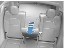
You can also fold the second row seat backs fully forward by pressing the corresponding switch located on the left side of the rear trunk area. Pressing the switch causes the seat back to swing forward. You can then push it downward so it lays fully flat.
