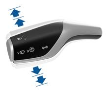
The turn signals stop operating when canceled by the steering wheel, by moving the lever in the opposite direction, or lightly pushing the lever in the same direction once more.
