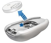
While avoiding touching the battery's flat surfaces, insert the new battery (type CR2032) with the '+' side facing up.
