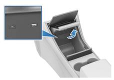
Two additional USB-C ports are located in the rear of the center console. Passengers in the rear seats can use these ports to charge their USB-connected devices. Devices connected to the rear USB ports do not communicate with the vehicle.
