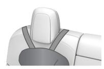
For a single-strap tether at an outboard seating positions, raise the head support (see Raising/Lowering the Outer Rear Seat Head Supports on page 30) and run the strap under the head support.
