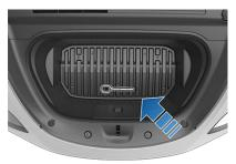
Release the front tow eye cover by pressing firmly on its top right perimeter until it pivots inward, then gently pulling the raised section toward you.
