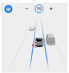
**Note:** To initiate Autosteer when there is no vehicle in front of you, you must be driving at least 18 mph (30 km/h) on a roadway with visible lane markings. If a vehicle is detected ahead of you, you can initiate Autosteer at any speed under 90 mph (150 km/h), even when stationary (if you are at least 5 feet (150 cm) away from the vehicle).
