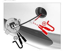
**Note:** Applying external 12V power to these terminals only releases the hood latches. You cannot charge the 12V battery using these terminals.
