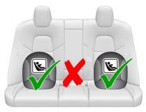
To install a LATCH child safety seat, slide the safety seat latches onto the anchor bars until they click into place. Carefully read and follow the instructions provided by the child safety seat manufacturer.
