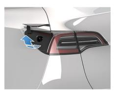
Note: The Tesla "T" lights up white when you open the charge port door. If you do not insert a charge cable into the charge port within a few minutes after opening the charge port door, the charge port door closes. If this happens, use the touchscreen to open the charge port door again
