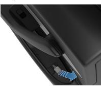
**Caution:** Manual door releases are designed to be used only in situations when Model Y has no power. Whenever Model Y has power, use the button located at the top of the interior door handle.
