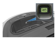
Press the interior release button to open the front trunk, then push up on the hood.
