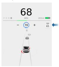
In situations where Model Y is unable to determine a speed limit, or if Speed Assist is uncertain that an acquired speed limit is accurate, the touchscreen may not display a speed limit sign and warnings do not take effect
