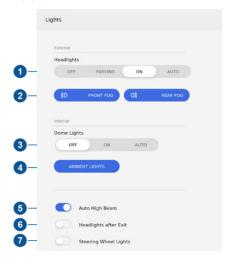
Exterior lights (headlights, tail lights, side marker lights, parking lights, and license plate lights) are set to AUTO each time you start Model Y. When set to AUTO, exterior lights automatically turn on when driving in low lighting conditions. If you change to a different setting, lights always revert to AUTO on your next drive.
