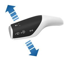
The high beam headlights can automatically switch to low beam when there is light detected in front of Model Y (for example. from an oncoming vehicle). To turn this feature on or off, touch Controls > Lights > Auto High Beam.
