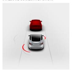
Warnings cancel automatically when the risk of a collision has been reduced (for example, you have decelerated or stopped Model Y, or the object in front of your vehicle has moved out of your driving path).
