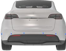
The sensors are activated when driving slower than 5 mph (8 km/h).
