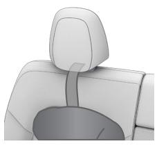
For a single-strap tether at the center seating position, raise the head support (see Raising/Lowering the Rear Center Head Support on page 30) and run the strap under the head support.
