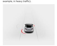
Lane Assist also warns you when a desired lane departure is not appropriate. When you engage the turn signal and a vehicle or object is detected in the adjacent lane you are planning to move into, the touchscreen displays a red lane line to indicate that a vehicle or object is detected. When the vehicle or object is no longer detected, the lane line returns to normal.
