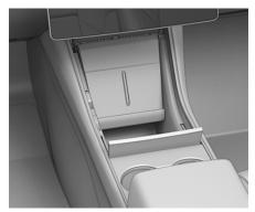
Model Y charges your smartphone only when the vehicle is powered on (i.e., the touchscreen is on, and you are in your vehicle). Your device will not continue to charge if you leave it plugged in after exiting the vehicle. Model Y will not charge your smartphone if the vehicle's Battery is discharged.
