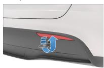
4. Attach the winch cable to the tow eve.
