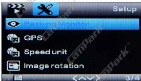
**Monitor di Parcheggio:** It's used to protect your car after parking, with this function on, after you stop the car and the camera turns off, it stays standby, when camera detects shaking, it will automatically turn on and take a short video, then shut down automatically.
